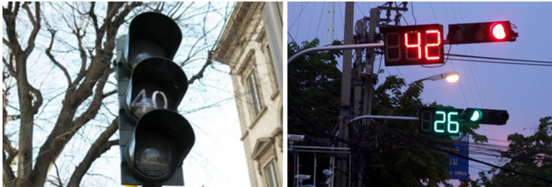
Figure 16 The hard priority granted to trams by the UTC system limits effectiveness of green wave corridors and countdowns at intersections.
